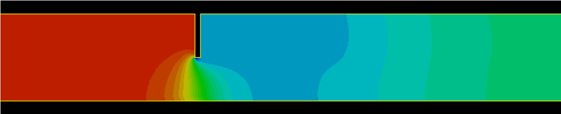
Figure 4.2: Contours of Static Pressure for Re = 40000
